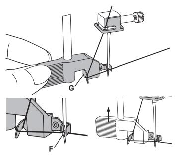
Note: When you are using a twin needle, you might need to reduce the stitch width to prevent damage of the twin needle, stitch plate or presser foot. How much you need to reduce it depends on the stitch position, the stitch width and/or the size of the twin needle.
