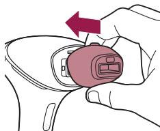
To remove the attachment, pull it off the light exit window.
